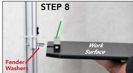
**Step 8:** Lift the Work Surface up and align the holes in the Horizontal Rail with the (2) 1/4-20 x 2.50 Hex Head Bolts{B}. Push the Work Surface onto the Hex Head Bolts until the threads of the bolts come through the Horizontal Rail.
