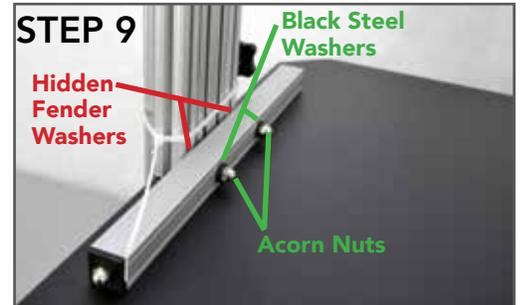
**Step 9:** Put (1) Black Washer{G} and (1) Acorn Nut{E} on the end of each of the Hex Head Bolts. Using the 7/16 wrench{H} tighten the Acorn Nuts securely. After you have the work surface secure, you can cut the zip tie holding the assembly together.
