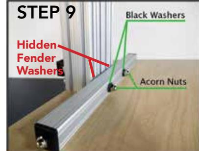
**Step 9:** Put (1) Black Washer{G} and (1) Acorn Nut{E} on the end of each of the Hex Head Bolts. Using the 7/16 wrench{H} tighten the Acorn Nuts securely.
