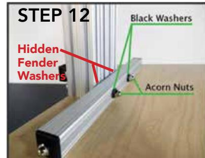
**Step 12:** Put (1) Black Washer{G} and (1) Acorn Nut{E} on the end of each of the Hex Head Bolts. Using the 7/16 wrench{H} tighten the Acorn Nuts securely.
