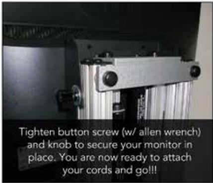
6. Tighten button screw (w/ allen wrench) and knob to secure your monitor in place. You are now ready to attach your cords and go!!!
