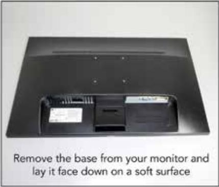
3. Remove the base from your monitor and lay it face down on a soft surface
