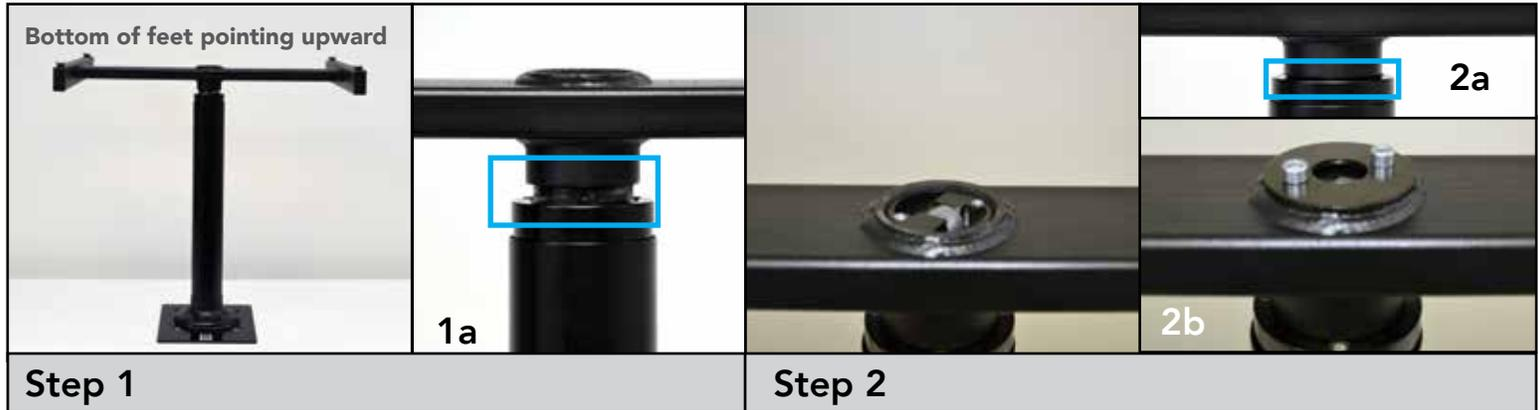
**Step 1: Attaching the H-Base.** Set the lifting column with the flat plate facing down. Place the H-Base on the column, feet facing upwards(as seen in #1). It will be a very tight fit. Make sure to twist and turn the H-Base left and right while pushing down to slide it on. It should appear like photo #1a above with a small gap between the lifting column and H-Base.
