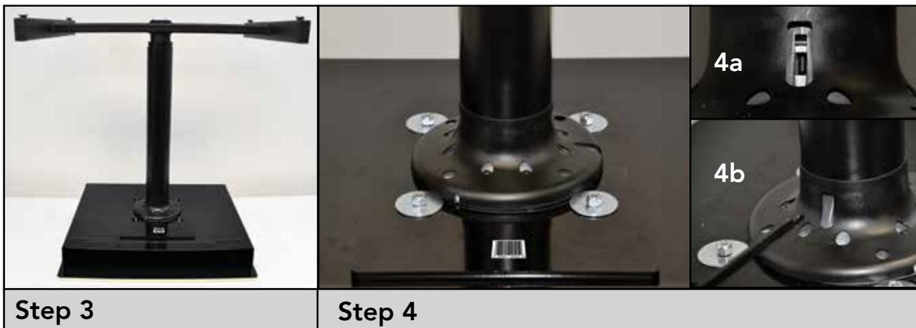
**Step 3: Attaching the desk basin to the lifting assembly.** Place the desk basin upside down with the open end facing you on a clean non-abrasive surface. Identify the (4) bolts on the bottom of the desk basin. Place the flat plate of the lifting assembly over the exposed desk basin bolts with the bar code sticker facing the opening of the desk basin. (See STEP #3)
