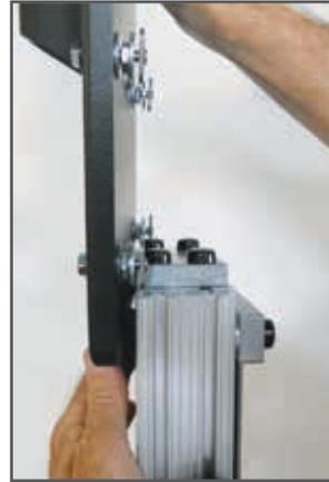
**Step 14:** Utilizing the monitor vertical rails from step 12, slide the backer board into the rails with the e-nuts on the back side.
