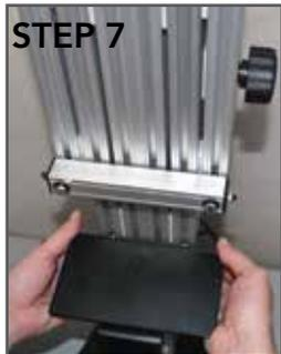
**Step 7: Installing the electric switch (DPG1C) and phone tray.** After the base has been attached, prep the tray by unscrewing the e-nuts until they are on the end of the bolt. Slide the tray on using the vertical channels of the lifting assembly as shown. Slide the tray up about 2 inches (this can be changed at any time), and lightly tighten the two bolts with the provided allen wrench.
