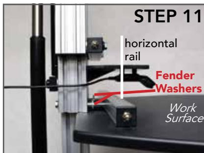
**Step 11:** Lift the Work Surface up and align the holes in the Horizontal Rail with the (2) 1/4-20 x 3.50 Hex Head Bolts{B}. Push the Work Surface onto the Hex Head Bolts until the threads of the bolts come through the Horizontal Rail.
